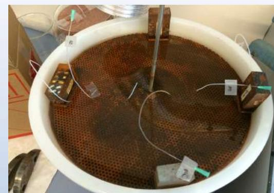
Sand saturated with water, contaminants (Ethanol and Dichloroethylene) have been added to the mixture.
